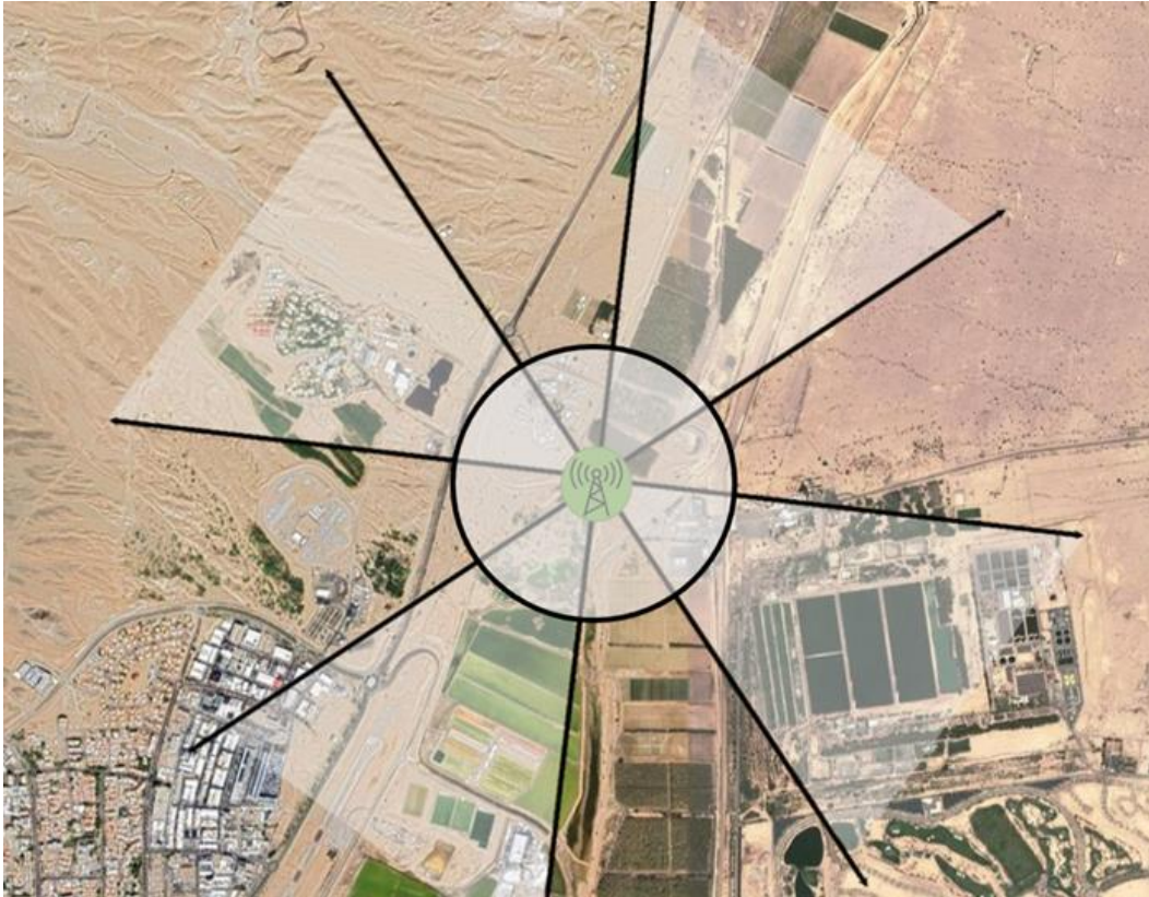
Fig. 1: Map with the receiver station at the IBRCE and the simplified coverage of the four directional antennas and one omnidirectional antenna.
